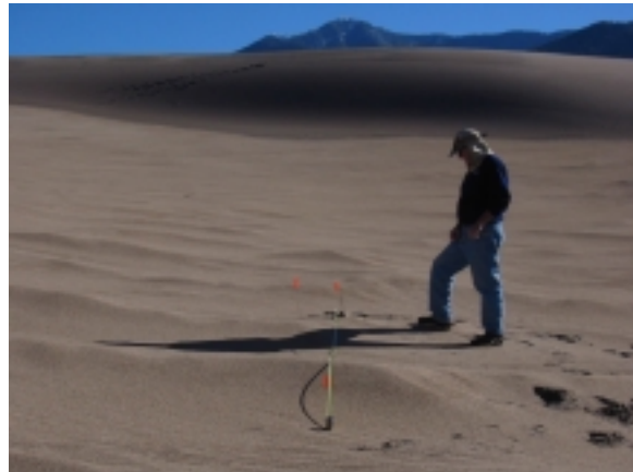
Figure 1. Laser profiling of granule ripples at Great Sand Dunes National Monument.
